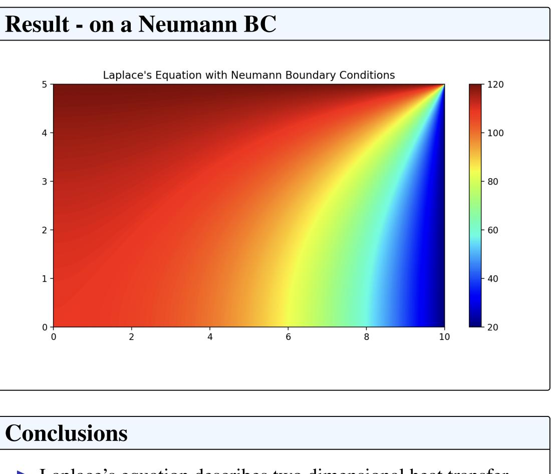
Laplace's equation describes two dimensional heat transfer ► The central difference method for second order derivatives is used to approximate the partial derivatives. ► If  $\Delta x = \Delta y$ , then each point in the grid is simply the average of the points surrounding it.
